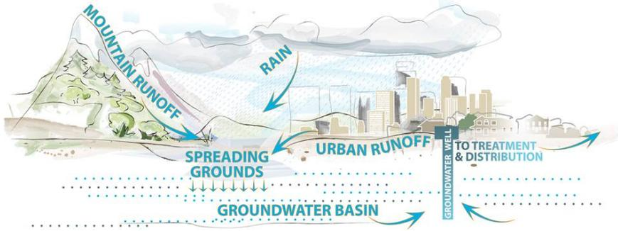
The stormwater capture projects come in various forms and may include catch basins, bioswales, pre-treatment devices, pumps, pump stations, storm drains, underground infiltration galleries, and other stormwater best management practices. Each project will be selected, sized and located within the park to maximize stormwater capture.
